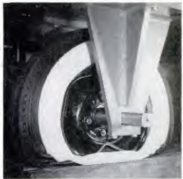
Despite 11 impacts at forces up to 23,000 pounds, the tire lost no air although wheel rim was bent
